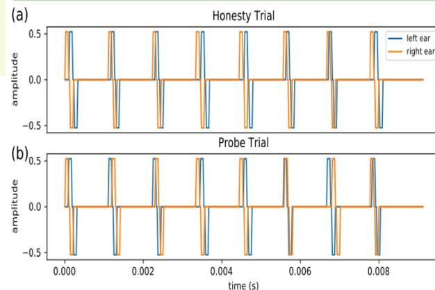
Figure 3: Examples of two trial types for electric biphasic pulse trains at 900 Hz delivered to CIs. (a) Honesty trial with only right leading ITDs with random jitter per pulse. (b) Probe trial with jitter jumping randomly between left and right leading ITDs. Amplitudes are relative to 100 µA at 0dB.
