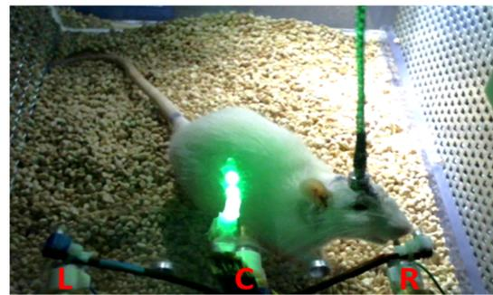
Figure 2: Setup for training bilateral CI-implanted rats on Z AFC binaural discrimination task by presenting ITD pulse trains directly to CIs. Three solenoid valves (L,C,R) with capacitance detector. Rat licks a computer interface and triggers release of water when response is correct. Incorrect responses results in a timeout.
